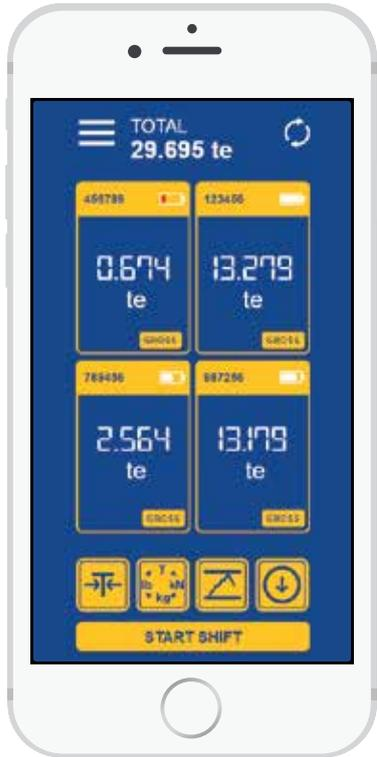
Up to four Crosby Straightpoint, Bluetooth load cells can be connected and monitored by up to eight smartphones, with the HHP2 app installed. It will enable more than one lifting professional to monitor the loads progress and safety, spotting potential dangers or issues from different vantage points.
