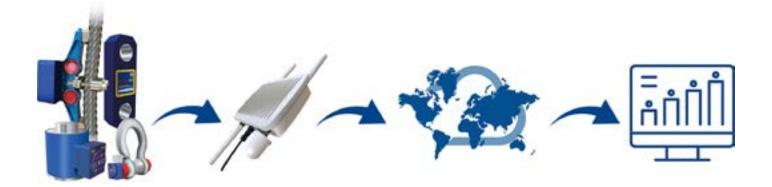
Base station WiFi (Part: LCBS-W) wirelessly connects to Crosby Straightpoint load cells or wire rope tension meter (BOLT) transmitting load cell load data and alerts via the local WiFi network to the LoadConnect online dashboard.
