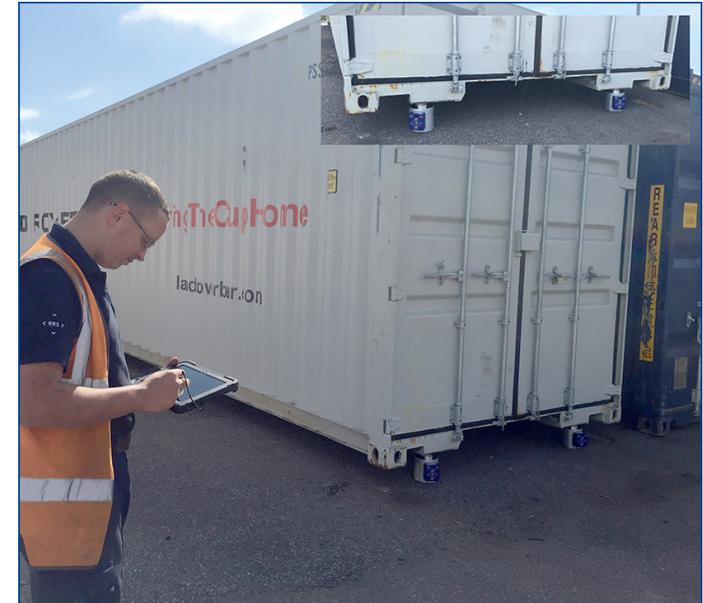
Plot the distances between your load cells in the grid template in the software.
