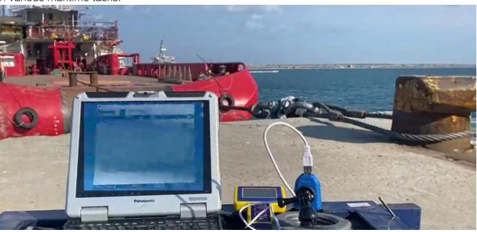
Crosby Straighpoint Radiolink plus with INSIGHT software and a handheld. *Note: Software distance is up to 700m, close proximity only for photographic purposes.*
