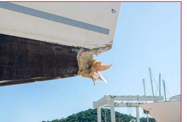
Damage to a ship after a bollard overload failure
