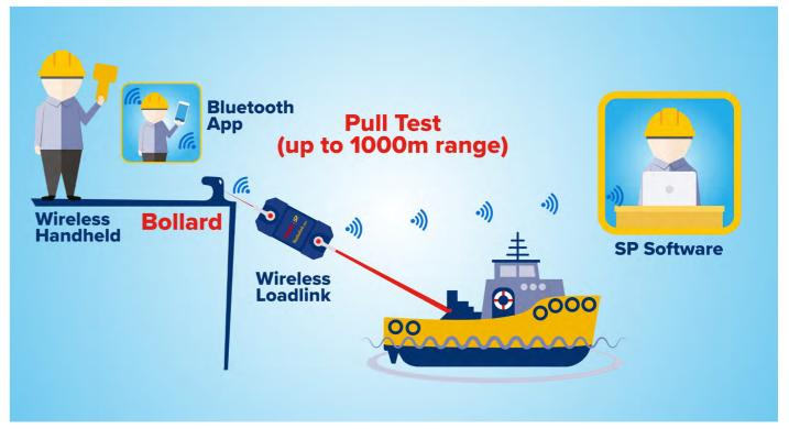
Bollard load testing and bollard pull testing for tugboats
