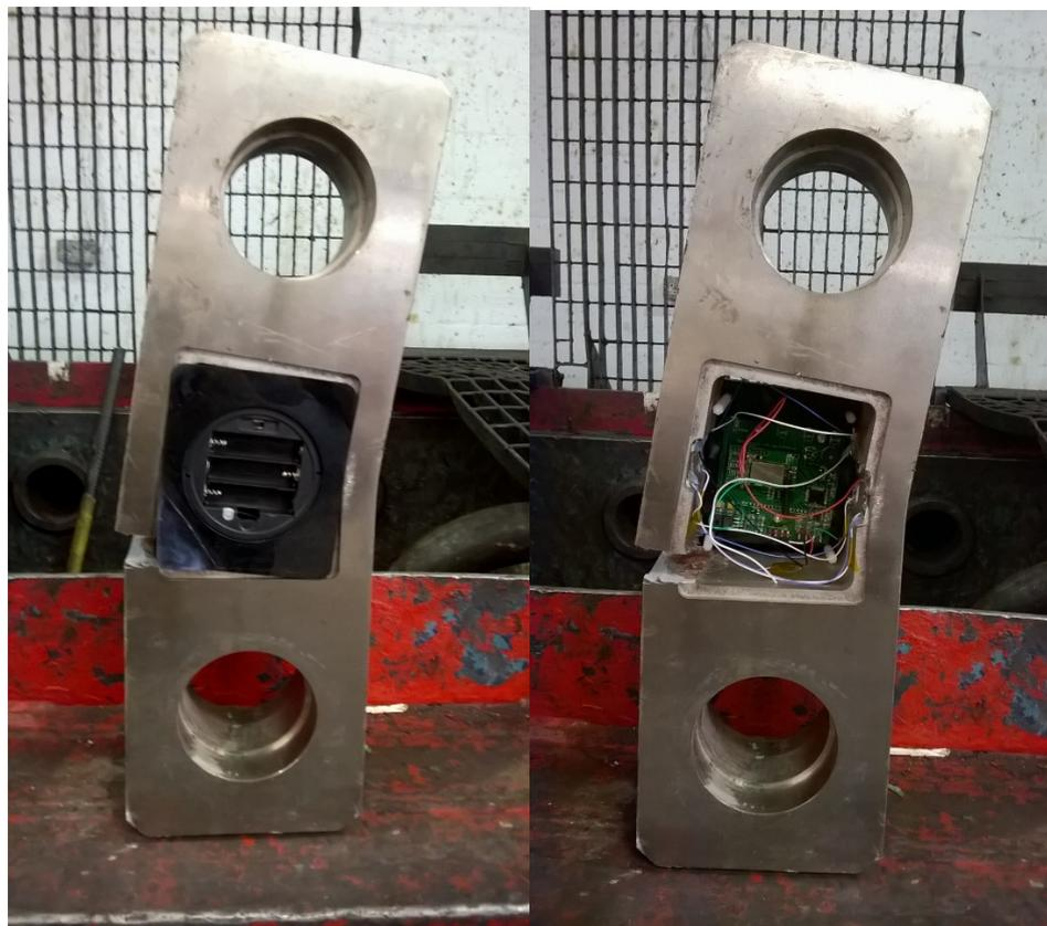
Photos of the load cell after it has yielded in the destruction test. As you can see it has snapped only on one side, which is highly unusual:
