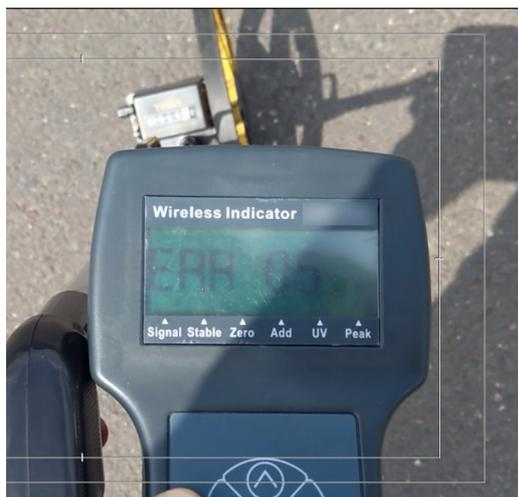
Figure B – Showing test setup with handheld being walked away from load cell by tester
