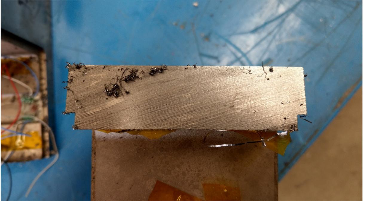
**Top down close up shot of the side that snapped in the destruction test**
