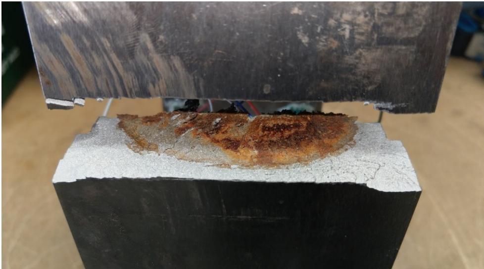
**Top down close up shot of freshly cut through side that did not snap in the destruction test**
