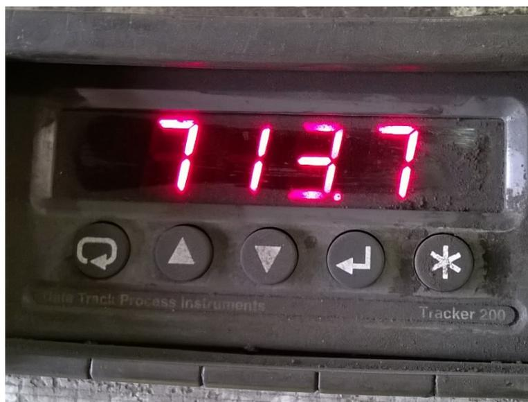
**Destruction test machine's reading at the point where the load cell snapped (71.37te)**
