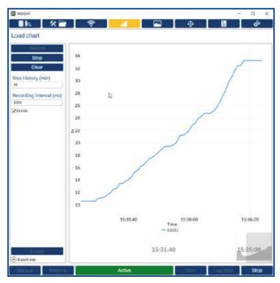
The main chart display shows this graph icon in the window, this graph is a constantly moving time line of the data at the current time.
