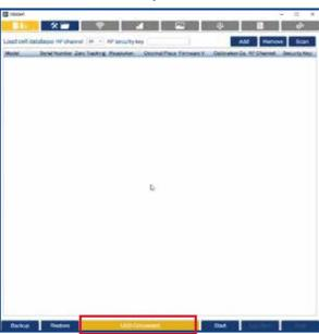
Note: If the USB dongle has been correctly inserted, the screen should show 'USB Connected' in amber at the bottom.
