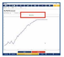
The on-screen graph will now populate with data as the test progresses, and at the same time, the live read window will show a live spot load reading.
